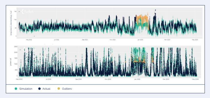
In addition, the turbine's output intermittently varied between 2300kW and 1185kW since October 24th and was continuously throttled to 1185kW from December 19th, 2022 on.
