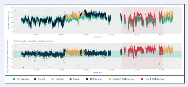
In response on 30th November, OEM confirmed that the main bearing was slightly damaged and initiated the necessary processes to organize the replacement the main bearing within the scope of a main component exchange action in the next five months. A flushing of the main bearing was performed and an additional second grease pump was installed to prevent further damage to the main bearing.
