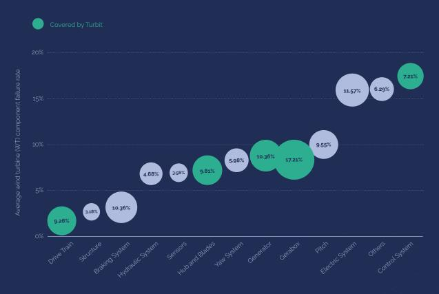
Turbit covers gearbox, generator, drivetrain and some power problems.
